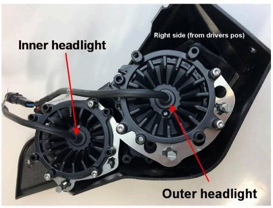
Use a 4 mm allen key (or simular) while doing the adjustments on the RJWC replacement brackets so that the plastic tabs don't slide out of position
